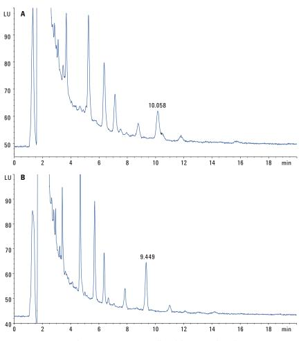
Figure 4. Determination of ochratoxin A in roasted coffee. A) Column 1: 4.6  $\times$  150 mm, 5  $\mu$ m. B) Column 2: 3.0  $\times$  150, 2.7  $\mu$ m.
