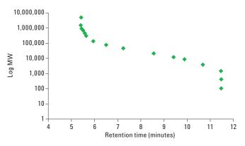
Figure 3. Polyethylene glycol and polyethylene oxide calibration curve using an Agilent Bio SEC-3, 300Å column.
