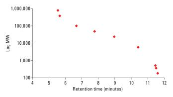
Figure 1. Pullulan polysaccharide calibration curve using an Agilent Bio SEC-3, 300Å column.
