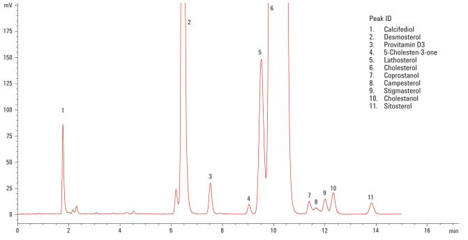
Figure 2. Separation of the sterol mixture (the ratio of cholesterol to other sterols was 2000:1) on an Agilent Poroshell 120 EC-C18, 3 × 100 mm, 2.7 µm column with evaporative light scattering detection.
