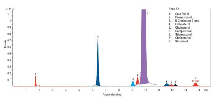
Figure 3. Separation of 9 sterols (the ratio of cholesterol to other sterols was 2000:1) on an Agilent Poroshell 120 EC-C18,  $3 \times 100$  mm, 2.7 µm with LC/MS/MS.
