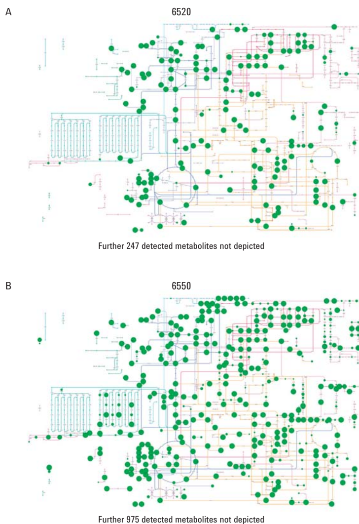
Figure 3. This map reports the compounds found by annotation and demonstrates six to seven times greater coverage with the Agilent 6550 Q-TOF (B) as compared to the 6520 Q-TOF (A). Dot sizes scale with the degree of confidence for the annotation.
