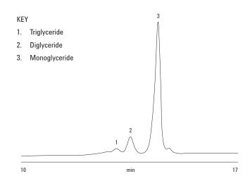
Three glycerides in a frying fat separated by Agilent PLgel 5 µm Figure 1. columns.
