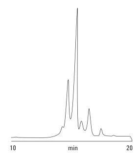
Figure 1. Separation of oligomers of a carboxylic acid ester on an Agilent PLgel 3 µm MIXED-E two-column set.
