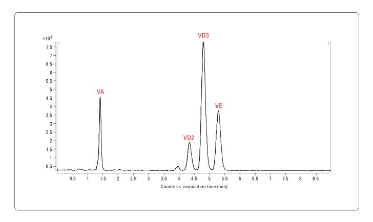
Figure 2. TIC of four fat-soluble vitamins on an Agilent ZORBAX Eclipse PAH column.
