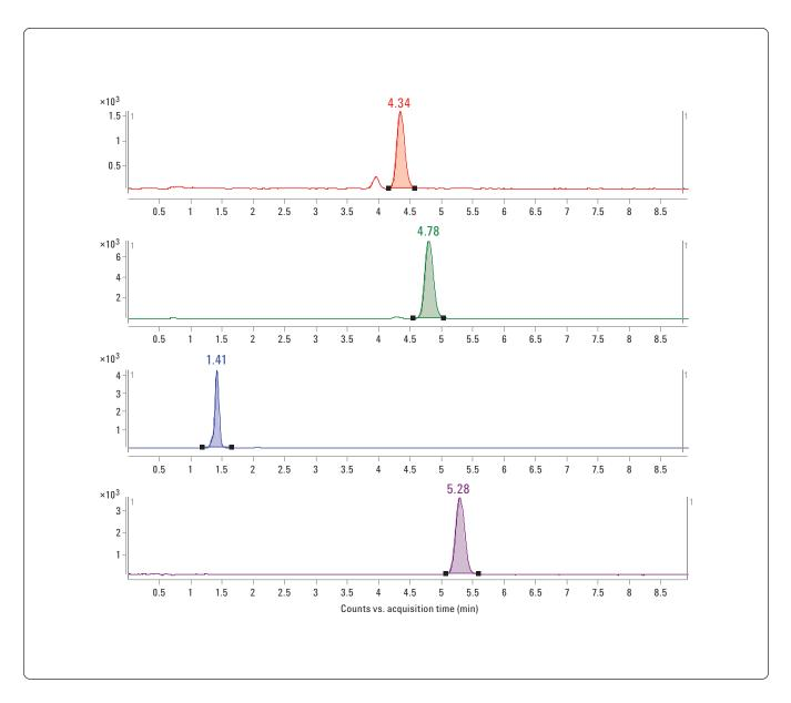
Figure 3. MRM of four fat-soluble vitamins on Agilent ZORBAX Eclipse PAH column.
