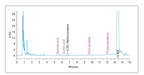
Figure 5 Chromatogram of a toothpaste.
