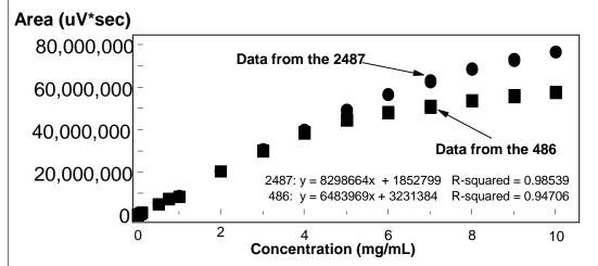
The following graph illustrates the concentration subset from 0.0005 mg/mL to 5 mg/mL from the previous linearity plot. Note the improved correlation coefficient calculated for the Waters 2487 detector.
