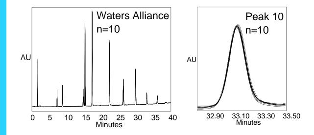
**Conditions:** Column: Symmetry® C18, 3.9 x150mm, 30°C; Flow rate: 1 mL/min; Mobile Phase: A=water, B=acetonitrile, both with 0.015% H3PO4; Gradient 0-80%B, 40 min, linear, vacuum degasser on normal; Detection: 254 nm; Sample: Gradient test mix
