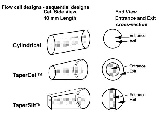
A typical cylindrical flow cell transmits the light inefficiently because some light hits the flow cell walls and causes refractive index (RI) effects. The **TaperCell™** technology increases the transmittance of light and reduce the RI effects by making the cell exit larger than the entrance, reducing the detector noise. The entrance of the cell allows for an eight nm bandwidth.
