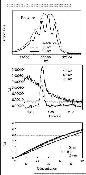
Optical resolution will determine the amount of detail observed in spectra. Benzene illustrates the spectral fine structure that can be seen at 1.2 nm resolution compared to 3.6 nm. 1.2 nm resolution is also required to distinguish between very similar compounds. For the highest quality spectral information which provides confident peak identification, the best optical resolution is required.
