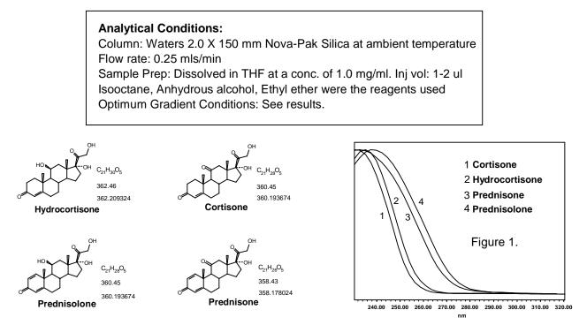
These chemically similar corticosteroids do not yield unique UV spectra (Figure 1.). Therefore, selective detection based upon unique chromophores for each compound is not possible.
