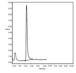
The following illustrates the reverse search capabilities of Palisade's PBM algorithm. The chromatogram to the right shows a perfect coelution of two benzodiazepines by flow injection of the compounds with no column in line. We then searched a "mixed' mass spectrum of the flow injected peak.
