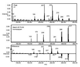
Positive compound identification of minor impurities is easily achieved using the Integrity LC/MS System. Simultaneous acquisition of PDA and MS data on a single injection and seamless processing and reporting of both channels of data as well as automated library search capabilities offer confidence in peak identification.
