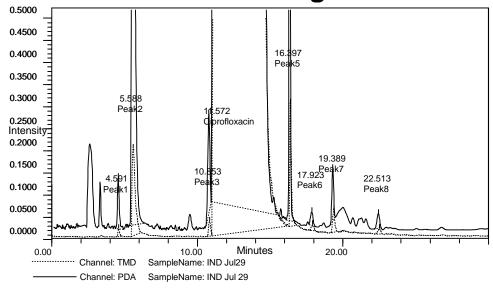
The ability to overlay PDA and MS chromatograms is unique to the Integrity System. Note there is almost no loss of chromatographic resolution when going from the PDA detector through the ThermaBeam mass spec interface. Both UV spectra and mass spectra can be acquired for each peak from the same sample injection and these can be used for compound identification.
