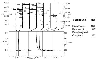
Positive identification of minor impurities is easily achieved using the Integrity LC/MS System. Simultaneous acquisition of PDA and MS data on a single injection and seamless processing and reporting of both channels of data as well as automated library search capabilities offer confidence in peak identification. In this example, Millennium Spectrum Index Plot displays the PDA and MS spectra of each chromatographic peak for powerful visual inspection and comparison of data.
