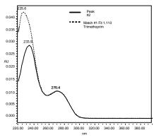
This represents the overlay of the UV Spectrum of the Unknown with the UV Spectrum of Trimethoprim.
