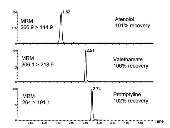
Representative LC/MS/MS data. Recoveries are the SPE recovery for rat plasma samples on the Oasis® WCX µElution plate. Excellent recoveries are obtained for all three classes of bases on this material.
