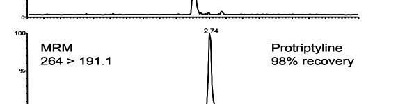
Representative LC/MS/MS data. Recoveries are the SPE recovery for rat plasma samples on the Oasis® MCX µElution plate. Excellent recoveries are obtained for both atenolol (polar base) and protriptyline (hydrophobic base). However, valethamate (quaternary amine) is retained on the sorbent.
