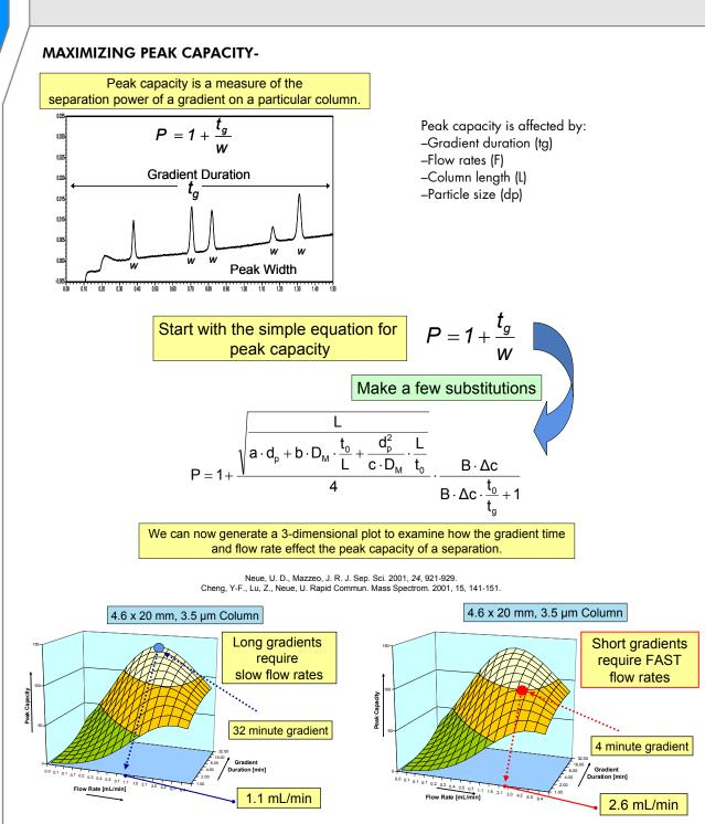
We see above that for a 32 minute gradient run on a 4.6 x 20 mm  $IS^{TM}$  column, a flow rate of 1.1 mL/min is predicted to maximize the peak capacity. But, for a 4 minutes gradient, a fast flow rate of 2.6 mL/min is predicted for maximum peak capacity.
