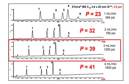
Recommended starting flow rates, to be adjusted according to the separation.
