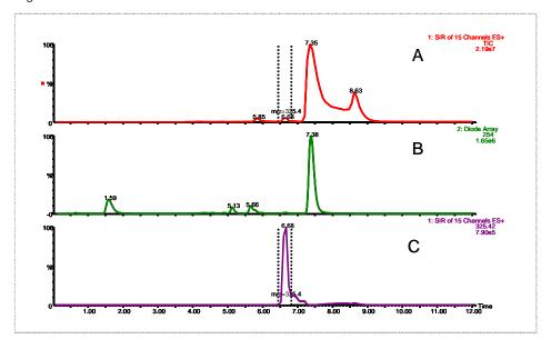
We then made a 20  $\mu$ L injection of the collected fraction. A) Total ion chromatogram. B) UV at 254 nm. C) Extracted chromatogram of m/z 325.4.
