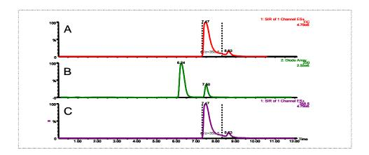
We then made a 20  $\mu$ L injection of the collected fraction. A) Total ion chromatogram. B) UV at 220 nm. C) Extracted chromatogram of m/z 358.5. We successfully collected 1.5 mg into one 2-mL well of the plate.
