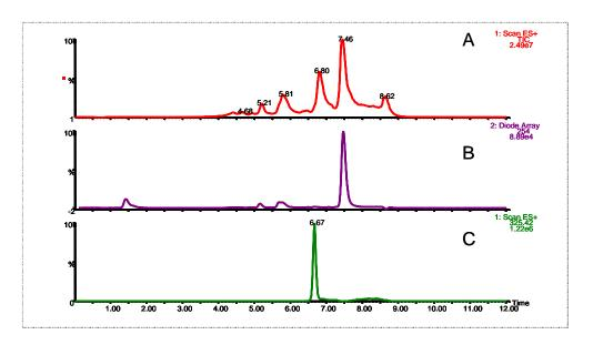
We set up the mass spectrometer to trigger collection using m/z 325.4. We then made an 800  $\mu$ L injection of the sample. A) Total ion chromatogram of 15 SIR channels. B) UV at 254 nm. C) Extracted chromatogram of m/z 325.4. Dashed lines indicated fraction collected.
