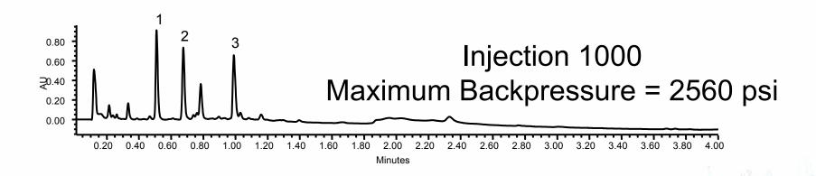
1000 injections on a 2.5 µm particle column with only a slight increase in backpressure!
