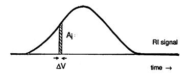
The concentration of sample in the column effluent at any slice in the polymer region of the RI response can be calculated using the RI data as follows:
