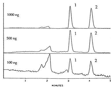
In order to obtain these detection limits, it is also necessary to minimize baseline drift. In contrast to noise, which remains at a constant level in a properly functioning detector, the amount of drift can vary widely and is often related to factors under the control of the operator. The Waters 410 provides the necessary detector control to reduce drift to the lowest possible level.
