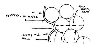
FLOW THROUGH A RADIALLY-COMPRESSED CARTRIDGE. SINCE THE BED IS TIGHTLY PACKED, BAND SPREADING DUE TO EDDY DIFFUSION IS GREATLY REDUCED AND EFFICIENCY IS HIGH.
