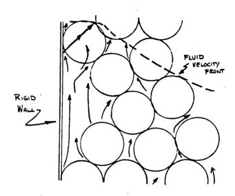
FLOW THROUGH A STANDARD STEEL COLUMN PRODUCES BROAD SAMPLE BANDS.
