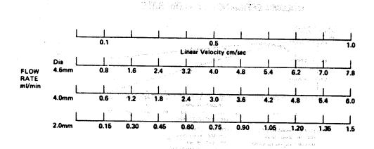
For the proper determination of linear velocity, it can be calculated from each column by the equation:  $u=L/t_m$  where u is the linear velocity, L is the column length and  $t_m$  is the time for the unretained peak.
