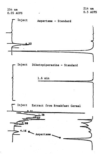
Conditions: Mobile Phase:  $\mu BONDAPAK^{TM}$   $C_{18}$  cartridge in Z-Module  $^{TM}$  25:CH\_3CN, 75:H\_2O + low UV PIC  $^R$  B-7
