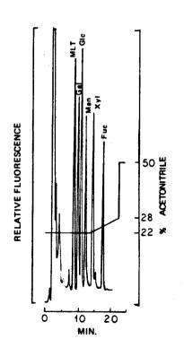
Chromatographic separation standard sugar-dansyl hydrazones. Conditions for separation described in text. Detector was Schoeffel FS970 Spetrofluoro Monitor (excitation wavelength, 240 nm; emission longpass filter, 550 nm; range, 0.2 sensitivity, 42%; time constant, 2.5 sec). Sample was 1 nmole each mlt, standard: maltose: galactose: glc, glucose; mannose; xyl, xylose; fuc, fucose.
