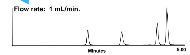
Column: Symmetry® C<sub>18</sub>, 5 µm, 4.6 X 50 mm Mobile phase: A=0.1% TFA in water, B=0.1% TFA in acetonitrile Gradient: 0-60% B in 4 minutes Column temperature: 30.0 °C Detector: 254 nm Injection volume: 1 µL
