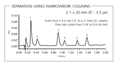
We can save further on the solvents by running the separation on a 2.1 mm I.D. column. We scale the flow rate to 0.6/ml. We can do the calculations for the shorter column and now have negligible costs in solvents — a savings of over \$2000!
