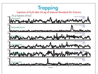
After analyses with 500 pg of each mixture component on column, an injection containing only the internal standard was made followed by an injection of  $\rm H_2O.$ A small amount of carryover for amitriptyline and propranolol was evident in the injection containing the internal standard. However, in the next injection consisting solely of H<sub>2</sub>O, the carryover was dramatically reduced.
