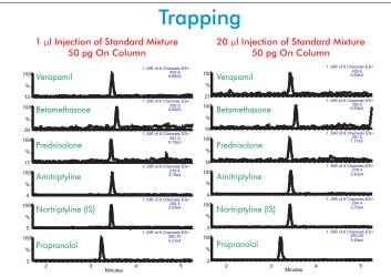
With these particular molecules, good separation was maintained when large volumes of the drug mixture were directly injected. Although trapping these molecules yielded some band broadening, the trapping configuration afforded the opportunity for on-line sample clean up.
