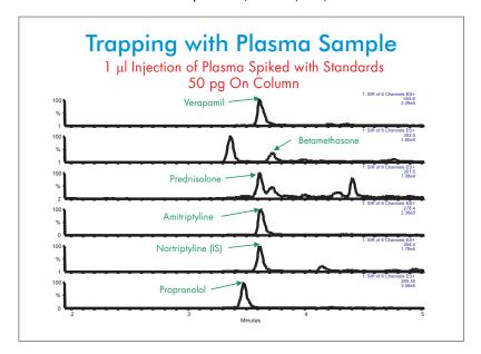
Plasma, diluted 1:1 with standards and IS in H<sub>2</sub>O, was loaded onto a trapping column for on-line sample clean up. After rinsing the proteins from the sample on the trapping column, the drug molecules were eluted from the trapping column and separated. Although some peak broadening was seen, good signal to noise was achieved with 50 pg of each sample molecule on column (25 pg of IS).
