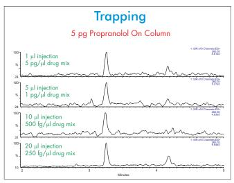
Similar sensitivities were attained for propranolol using direct injection and trapping methods.
