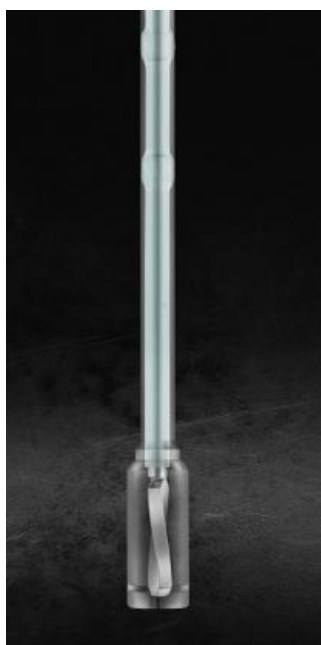
Figure 3. LV Nano ITC cell and paddle
