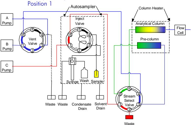
As the sample elutes from the pre-column, it is carried into the analytical column where separation occurs. By plumbing Pumps A and B into the stream select valve and by-passing the injection valve and loop, the system volume is significantly decreased which reduces the gradient delay time.
