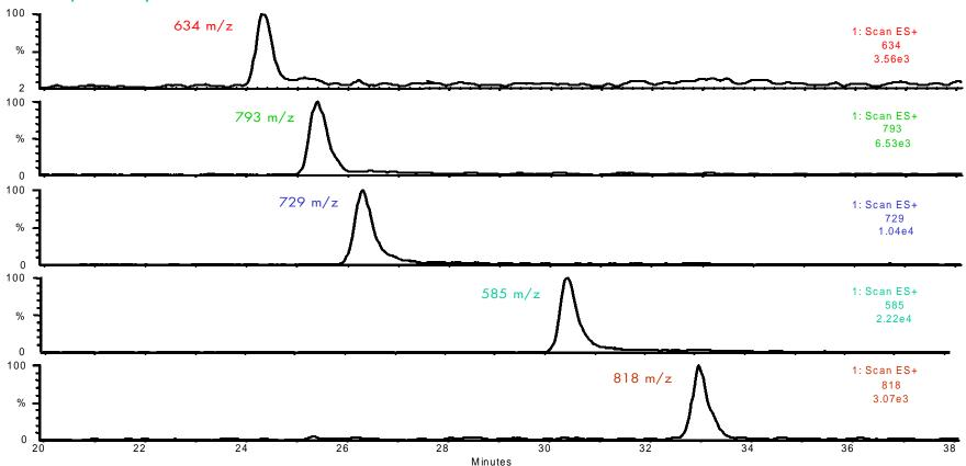
This separation was performed on a 180  $\mu$ m column with a flow rate of 2  $\mu$ l/min and a standard ESI source fitted with a 60  $\mu$ m i.d. capillary (microspray). The increased flow rate decreased the total run time for the analysis by 32 minutes. The use of a microspray ESI interface with a flow rate of 2  $\mu$ l/min yielded a signal comparable to that given by the nanospray source at 1  $\mu$ l/min.
