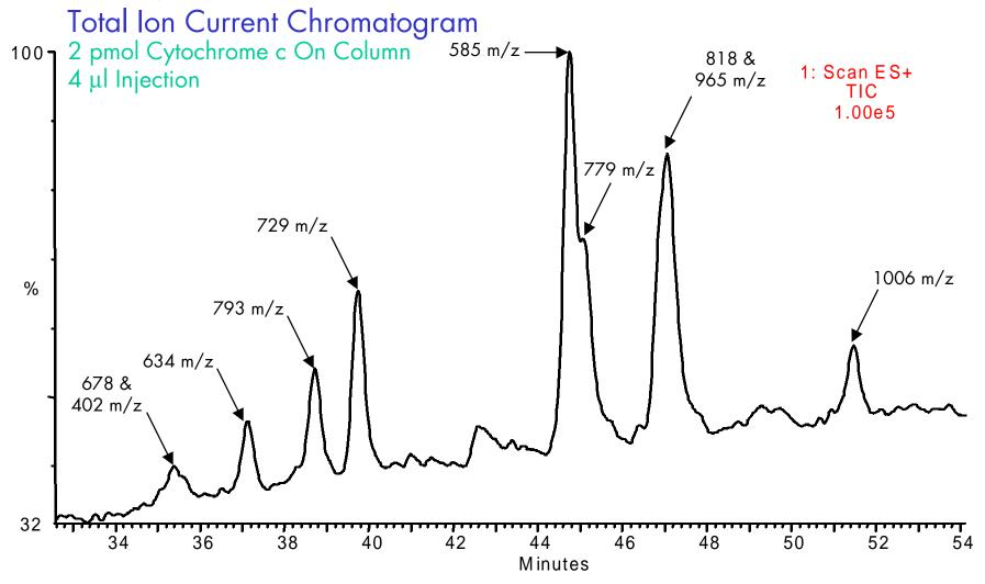
In this analysis,  $4 \,\mu l$  of a 500 fmol/ $\mu l$  sample solution were concentrated on the precolumn and then separated on a 180  $\mu m$  column. The ability to trap sample on a pre-column could be very useful in situations where large volumes of solution must be loaded to provide an appreciable amount of sample or in instances where on-line sample clean-up must be performed.
