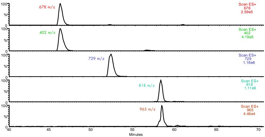
The ability to extract masses from a total ion current chromatogram allows for the resolution of coeluting peaks as shown above. While complete chromatographic resolution is favorable to minimize ion suppression in the source, peak resolution for identification and qualitative analysis of particular ions can be achieved by extracting masses of interest.
