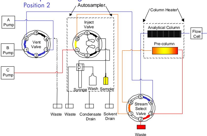
Sample is loaded onto the precolumn at a high flow rate using Pump C. Using an integrated six position valve, the sample is trapped on the precolumn, and the loading solvent is directed to waste. Once the sample has been loaded, the stream select valve changes positions and the sample is eluted from the precolumn with the gradient formed by Pumps A and B as shown below. In this instance, the pre-column is backflushed. © 2000 Waters Corporation
