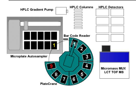
The layout of a typical automated HPLC-MS workcell is shown here.
