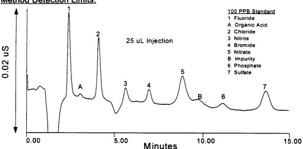
Based upon this representative chromatogram using a 25  $\mu$ L injection, the estimated detection limits, as ppb, at 3 times signal to noise (S/N) are:
