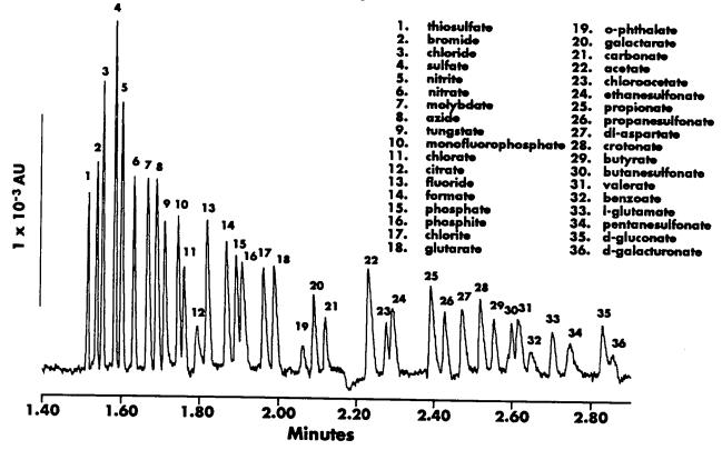
This is a recent anion separation illustrating the peak capacity of CIA methodology. The anions are in the 0.3 to 3.3 ppm concentration range. IC can do the same number of anions but requires 30 minutes and gradient elution.
