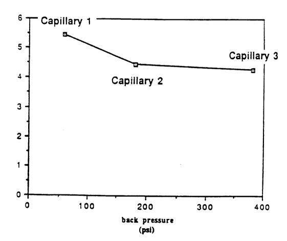
In order to determine the impact of the packing material on the rate of osmotic flow, 3 capillaries with dimensions of 100  $\mu$ m x 60 cm were tested. The pack pressure was determined using an HPLC pump with a flow rate of 100  $\mu$ l/minute. The rate of osmotic flow was determined using a neutral marker.
