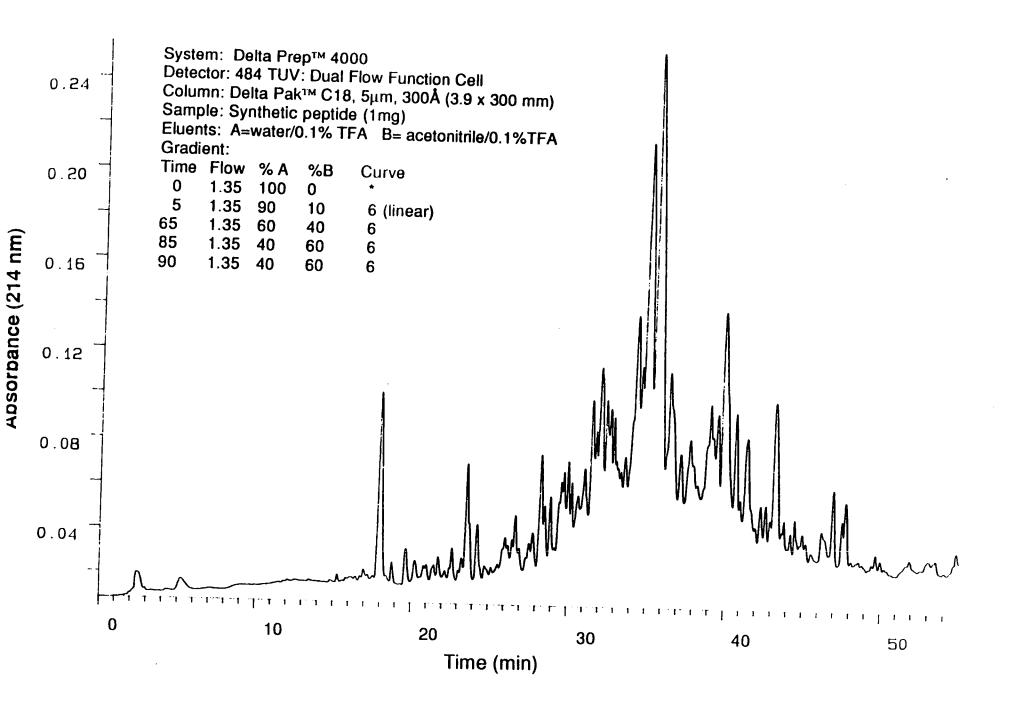
Figure 1 Small-scale Separation of 1mg Synthetic Peptide on 5  $\mu$ m Reversed Phase Support. The reaction mixture was separated on a small (3.9 x 300 mm) high resolution 5  $\mu$ m C18 column. An optimized gradient was developed to maximize the resolution of the peptide eluting at 35.4 min. Due to the complexity of this mixture, a multi-step approach to the purification was developed.
