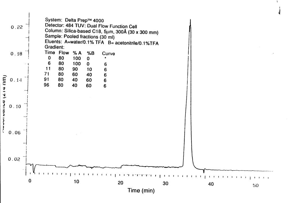
Figure 5 Large-scale Purification of Pooled Fractions on 5  $\mu$ m Support. The Pooled Fractions were purified on the preparative-scale with minimal loss of resolution. Fractions were collected and screened for purity by reversed phase HPLC.
