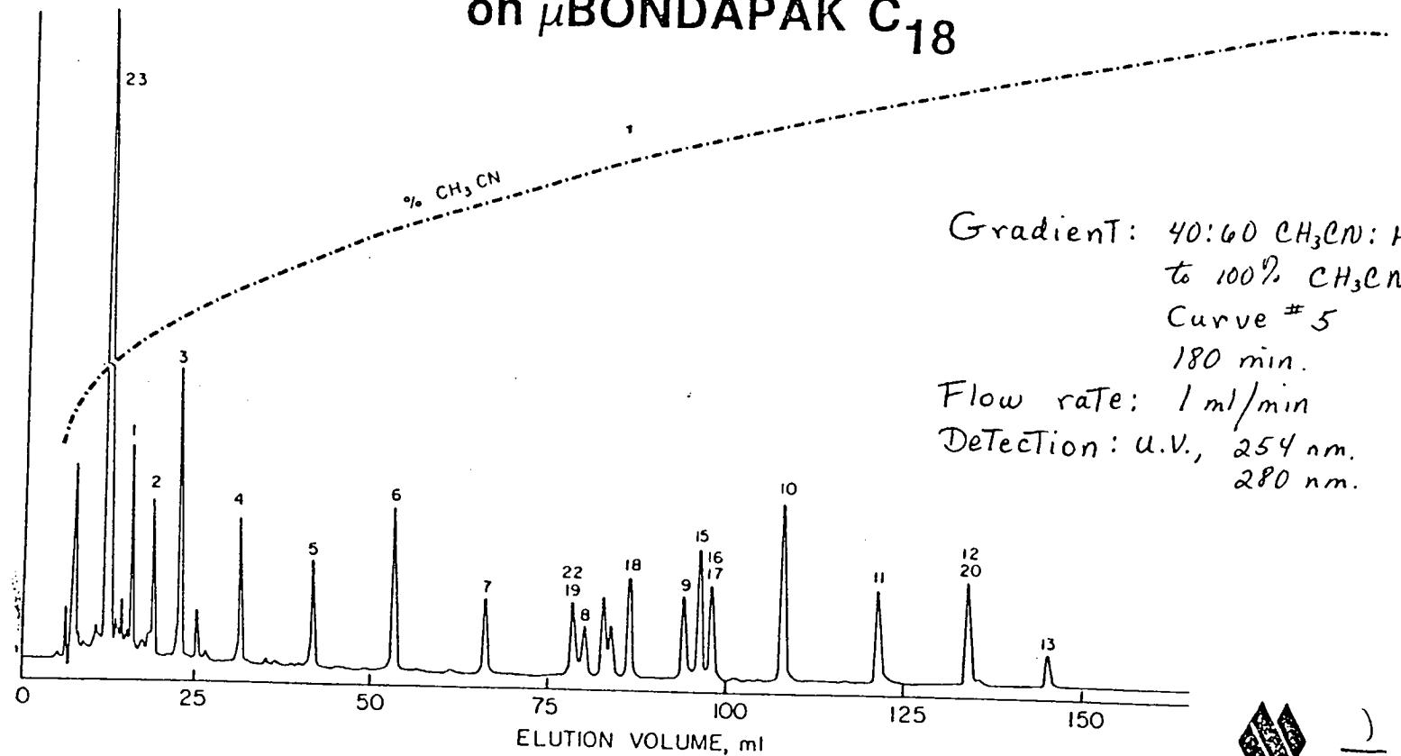
Five in a series of nine. The separation of *p*-nitrophenacyl esters of fatty acids, C<sub>2</sub> - C<sub>24</sub> saturated and unsaturated.
