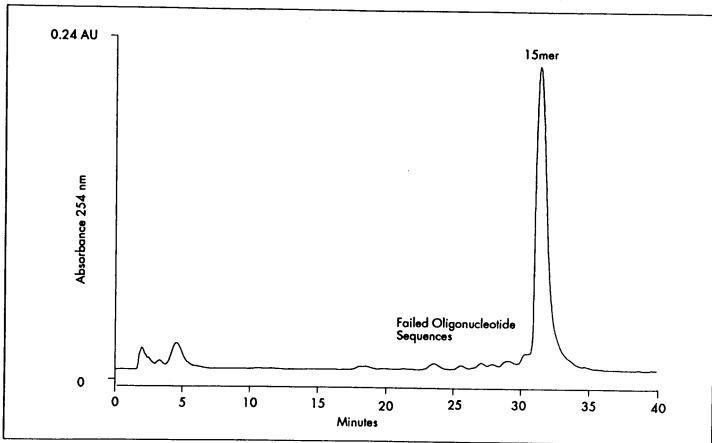
Cyclone Plus Synthesis of Oligonucleotide (15mer, random sequence); Fast Probe Protocol (FPP) 200nM
