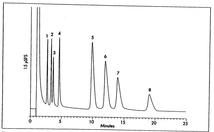
The Waters IC-Pak™ C M/D column allows for the simultaneous, isocratic separation of monovalent and divalent cations in only 20 minutes. Detection limits for most species shown are less than 10 ppb. This method is also applicable to the analysis of amines and alkanolamines
