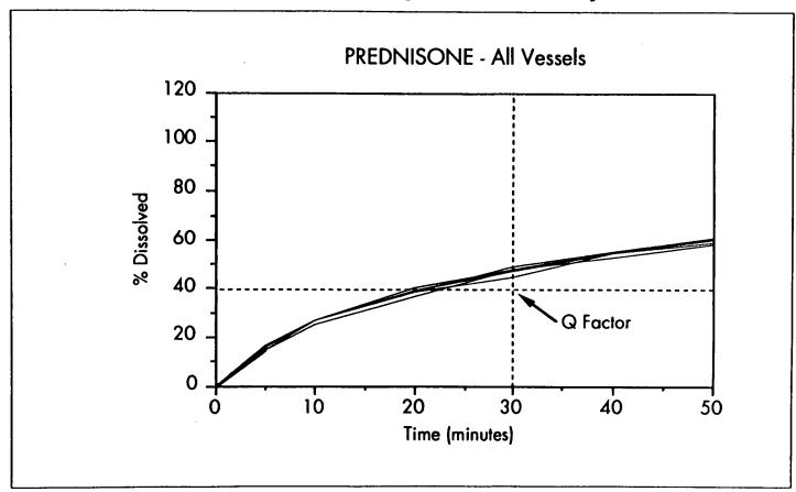
Waters Dissolution System automates the transfer of samples from the dissolution bath to the HPLC autosampler. The HPLC injects samples while the dissolution occurs, saving time. Post-run data reduction produces dissolution profiles, statistics and determines pass or failure of the dissolution test (Q-Factor).
