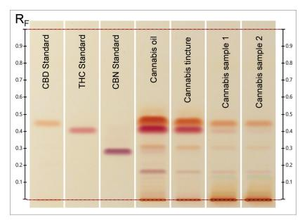
Figure 2. Derivatized HPTLC plate under white light (remission).
