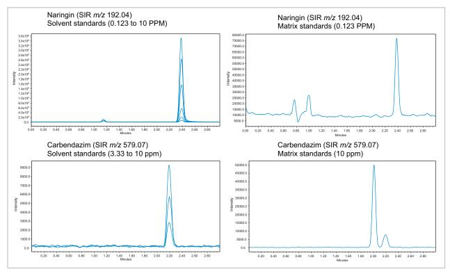
Figure 3. Overlay of solvent and matrix standards.
