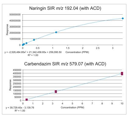
Figure 5. Calibration curve for solvent standards with ACD.
