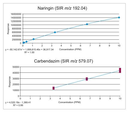
Figure 2. Calibration curve for solvent standards.
