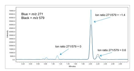
Figure 4. Overlay of ions.
