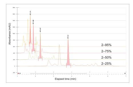
Figure 4. Results from the method scouting runs. The retention time of chlorogenic acid is shown in each chromatogram. A linear gradient was run for 5 minutes from 2% to 95%, 75%, 50%, and 25% organic concentrations, respectively.
