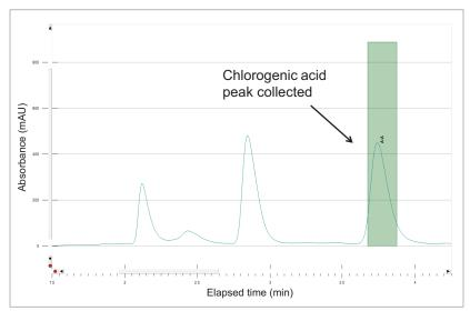
Figure 8. Chlorogenic acid peak collected at prep scale (19 mm  $\times$  50 mm) by absorbance threshold in the ChromScope Software.
