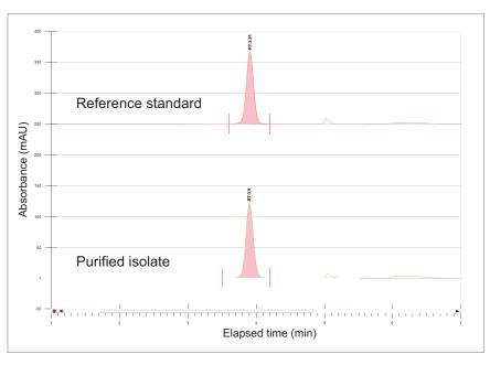
Figure 9. Overlay of the chlorogenic acid purified isolate (green) compared with a reference standard (red) analyzed by the focused gradient with the  $4.6 \times 50$  mm analytical column.
