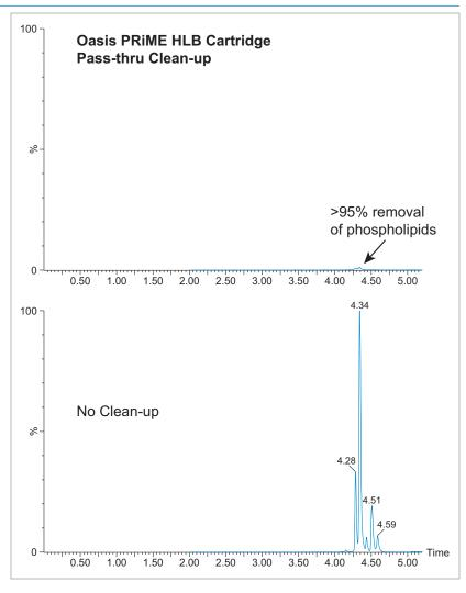
Figure 1. LC-MS/MS chromatograms showing effective removal of  $\geq$ 95% of phospholipids from shrimp extract.
