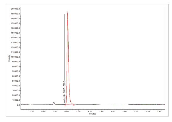
Figure 3. A chromatogram depicting 10 replicate injections of sample 1403736 on the UPLC-MS at 0.2 µL injection volumes. Retention time relative standard deviation (RSD) was 0.07% and area RSD was 1.2%. See Table 2 for concentrations.
