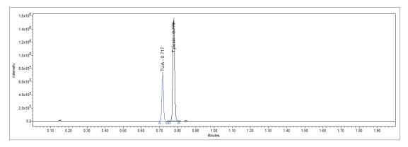
Figure 4. A chromatogram of sample 1403965 displaying m/z = 916.61 for Tylosin (black) and m/z = 1018.70 for TUA (tylosin + 2 urea –  $H_2O$ , blue) using UPLC-MS.
