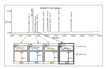
Figure 3. Confirming peak identity by mass detection using mass spectral data acquired with an ACQUITY QDa Detector. Mass analysis window from Empower 3 Software shows UV and mass spectral data from a single result.
