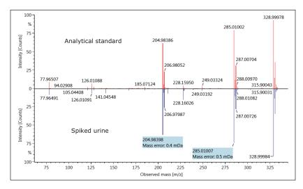
Figure 4. Results of the binary comparison analysis for furosemide (the plot is scaled to the relative percentages of the identified fragments). The data have been generated using the binary compare tool in UNIFI and highlight the mass error between the standard (upper-trace) and the sample data (lower-trace).
