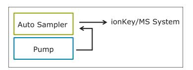
Figure 1. Instrument configuration for direct sample injection onto the ionKey/MS System.
