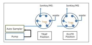
Figure 6. Instrument configuration using single pump trapping.
