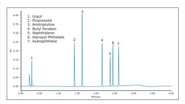
Figure 2. Reversed Phase QC Reference Material Chromatogram, using an ACQUITY UPLC CSH  $C_{19}$ , 1.7  $\mu$ m, 2.1 x 50 mm.
