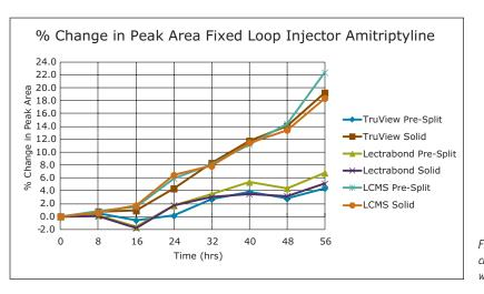
Figure 4. Amitriptyline peak area change using the fixed loop injector with different vial cap types.
